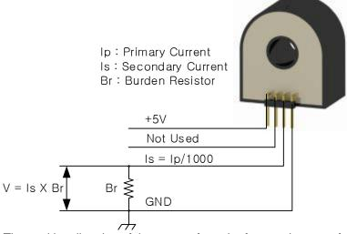
\* The positive direction of the current from the front to the rear of the head (the front of the contactor).
