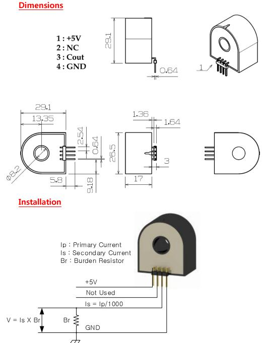
\* The positive direction of the current from the front to the rear of the head (the front of the contactor).
